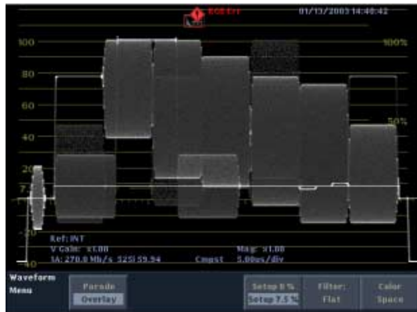
Figure 2-37: Waveform mode Overlay display showing the Composite graticule with 7.5% setup selected
